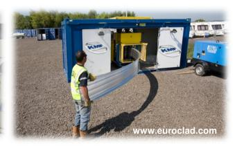
The CURVEmax can be located on site, it is contained inside a 20ft container and can produce single, multi and waveform curves on site down to a 1.5 metre radius. (minimum radii are depending on material specification)
